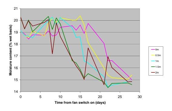
Figure 4. Moisture content of grain sampled at depths from 0 to 2.0m below the grain surface in Bin 6 against time.
