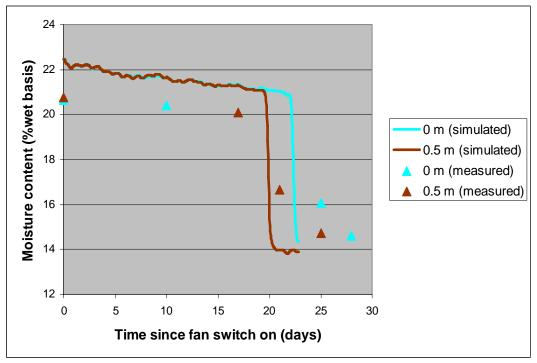
Figure 25. Predicted and measured moisture contents at the surface and a depth of 0.5 m for Bin 4 with 125% measured airflow.
