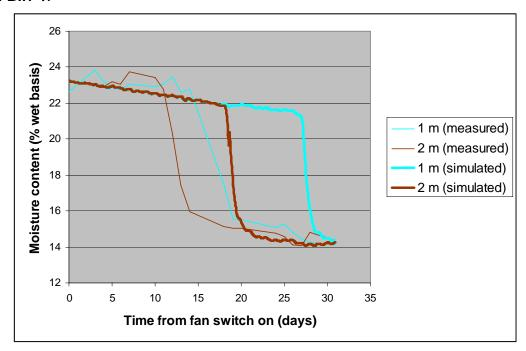
Figure 12. Measured and predicted moisture contents at depths of 1 and 2 m in Bin 5.
