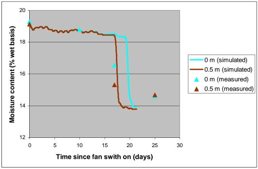
Figure 27. Predicted and measured moisture contents at the surface and a depth of 0.5 m for Bin 6 with 125% measured airflow.
