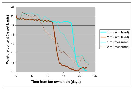
Figure 17. Predicted and measured moisture contents for depths of 1.0 and 2.0 m Bin 4 with 125% measured airflow.
