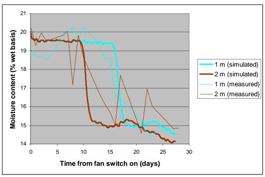
Figure 19. Predicted and measured moisture contents for depths of 1.0 and 2.0 m Bin 6 with 125% measured airflow.
