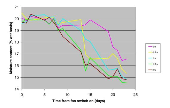
Figure 2. Moisture content of grain sampled at depths from 0 to 2.0m below the grain surface in Bin 4 against time.
