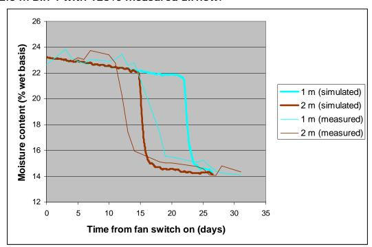
Figure 18. Predicted and measured moisture contents for depths of 1.0 and 2.0 m Bin 5 with 125% measured airflow.
