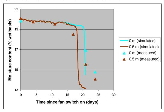
Figure 26. Predicted and measured moisture contents at the surface and a depth of 0.5 m for Bin 5 with 125% measured airflow.
