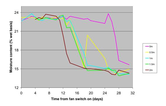
Figure 3. Moisture content of grain sampled at depths from 0 to 2.0m below the grain surface in Bin against time.
